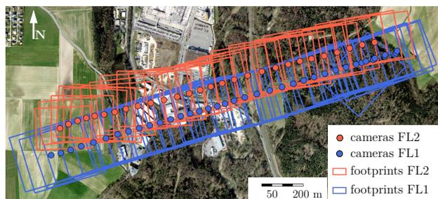
**Figure 3.** Overview of the study area and the image footprints for the flight lines (FL) studied. Both urban and rural areas are enclosed in the mapping area.
